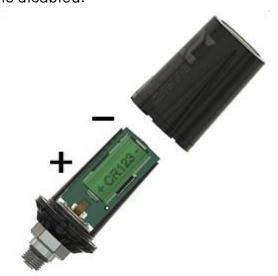
If the negative terminal of the battery is oriented toward the high-pressure port, the position data transmission is enabled.
