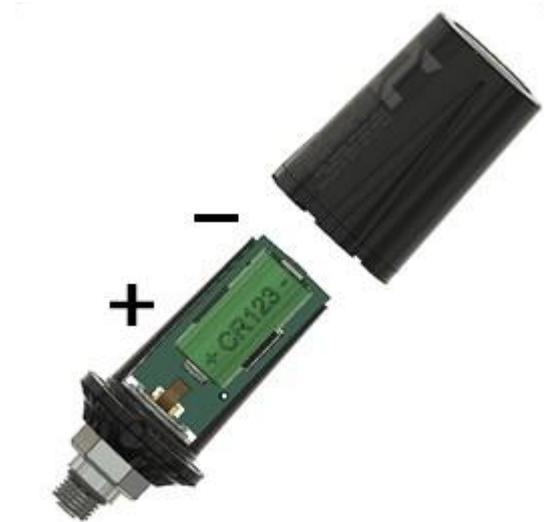
If the negative terminal of the battery is oriented toward the high-pressure port, the position data transmission is enabled.
